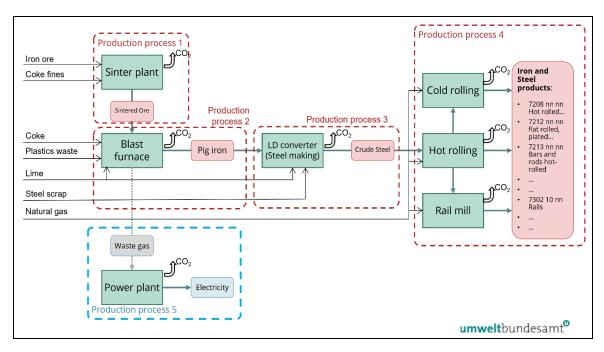
Direct emissions arise from the combustion of fuels (coke fines, plastic wastes, natural gas) and from the waste gas (blast furnace gas) used for power generation, and from process emissions from coke<sup>134</sup> as reducing agent and the thermal decomposition of carbonate-containing materials (such as lime) and from releases of carbon contained within the different iron and steel materials.
