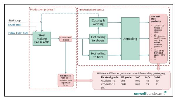
The two relevant production processes defined above, and elaborated further in the diagrams below are:
