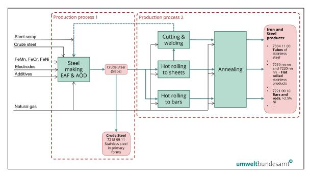
Direct emissions arise from the combustion of fuels (natural gas) and from process emissions from graphite electrodes, other additives and from releases of carbon contained within the different iron and steel materials.
