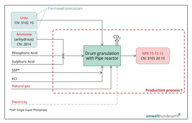
Inputs into the production process are raw materials, precursor goods urea and ammonia (anhydrous), and electrical energy. Outputs are mixed fertilizer product.
