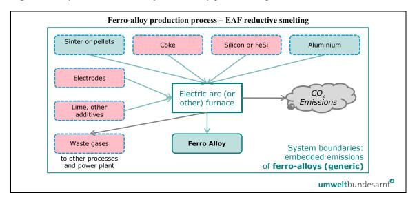
Note that raw material inputs for ferro-alloys may include pellets and sinter that are produced under the separate production process (for CN code 2601 12 00) for sintered iron ore.
