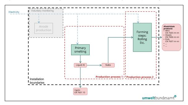
The fourth diagram (Figure 7-16) provides a complete monitoring approach for all source streams, for the example installation.
