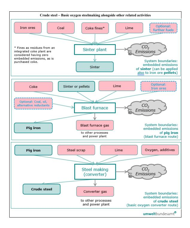
In integrated steel plants, liquid pig iron that is directly charged to the oxygen converter is the product which separates the production process for pig iron (bottom left in *Figure 5-11* above) from the production process of crude steel (bottom right, above).
