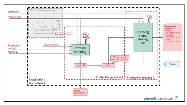
The inputs and outputs highlighted in red text in Figure 7-16 are the parameters that would need to be monitored by the operator in order to attribute emissions and determine direct and indirect specific embedded emissions for both production processes.
