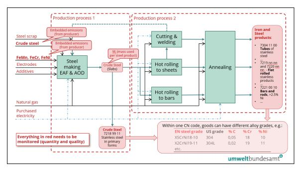
In iron and steel example 1 (section 7.2.2.1), a 'bubble' approach was used, as all precursors produced by the installation are wholly used in the production of the finished iron and steel goods. However, this approach is not available to the operator in this example, as some of the crude stainless-steel precursor produced by production process 1
