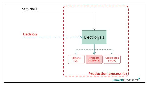
*Figure 7-18: Hydrogen example No.2 – Overview and complete monitoring approach for hydrogen*
