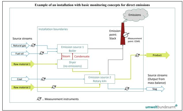
The fictitious example installation consists of a dryer in which raw material 1 is dried using steam from a boiler. This material is considered not to contribute to the emissions. Another
