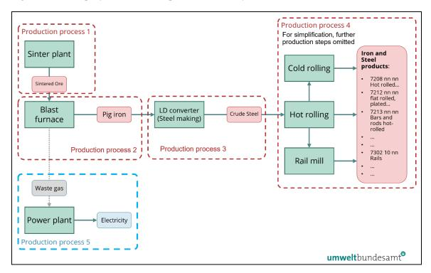
The five relevant production processes defined above, and elaborated further in the diagrams below are:
