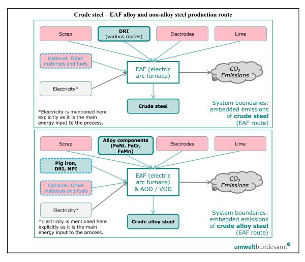
There are several different EAF production routes, for crude steel and crude alloy steel, which are broadly similar and are shown jointly in Figure 5-12.
