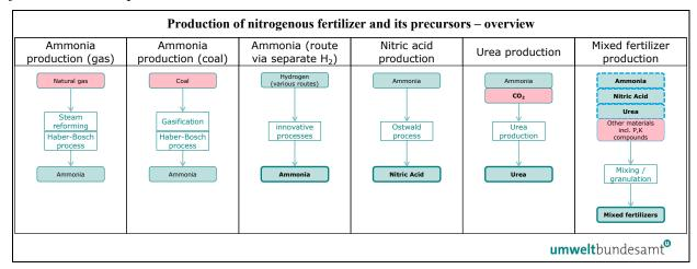
Urea is used as a precursor in mixed fertilizer production but may also be used as a convenient fertilizer on its own due to its high nitrogen content.
