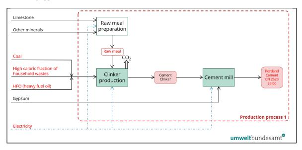
The system boundary has been redrawn to encompass both production processes previously defined for each CBAM aggregated good.
