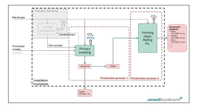
Direct emissions above result from fuel combustion in both production processes, and from the primary smelting process - from the consumption of carbon anodes and from the formation of PFCs.
