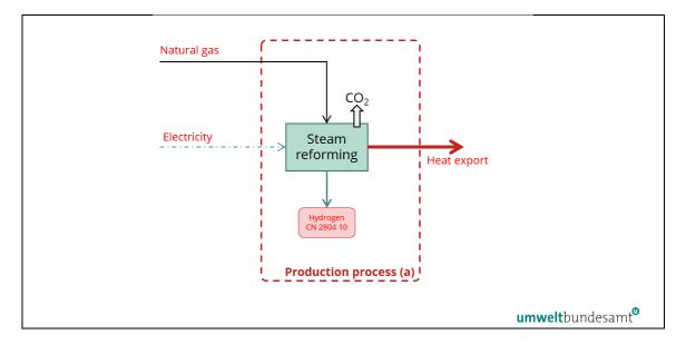
A single production process is defined for steam reforming. Inputs are natural gas (both as a raw material / feedstock for the process, and as a fuel) and electrical energy. Outputs are hydrogen product and heat exported to other parts of the installation or to a district heating network.
