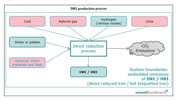
Figure 5-10: System boundaries of the DRI production process
