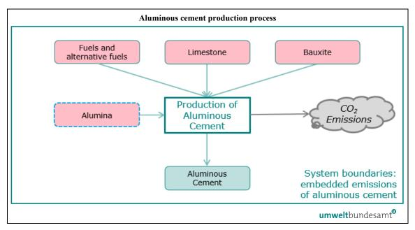
Note that alumina (produced from bauxite) is treated as a raw material and has zero embedded emissions.
