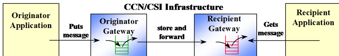
Figure 23: CCN/CSI asynchronous service
